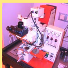
Masks alignment and insulator for UV- Photolithography
