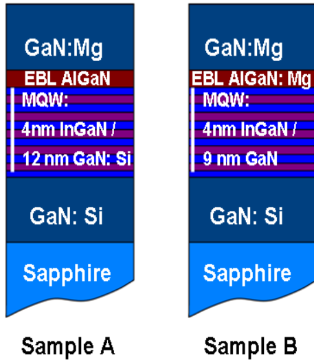
Figure 3. Reference and improved InGaN/GaN MQW heterostructures used in the optimization experiment.
